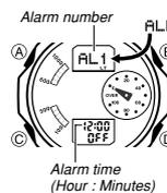
When an alarm is turned on, the alarm tone will sound when its alarm time is reached. One of the alarms is a snooze alarm, while the other four are daily alarms.
